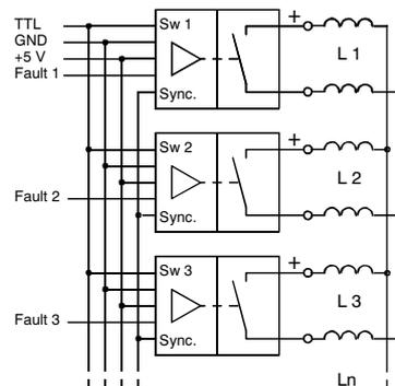
**Note:** Symmetrical layout is recommended for good dynamic current sharing (Wiring inductance  $L_1$  to  $L_n$  should be equal).
