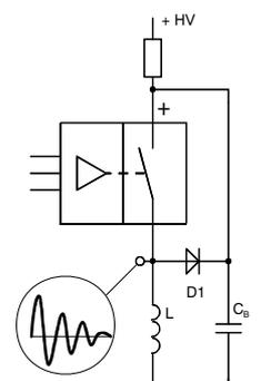
**Note:** D1 is a fast recovery diode with Kiloamps peak current capability (E.g. Behlke Series FDA)
