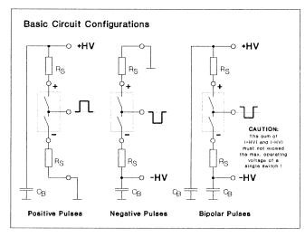
circuit in the bridge. For this reason inductive loads are permitted only when it is absolutely certain that there can be no current direction reversal, e.g. by building in fast series diodes and/or by using RC snubbers or clamping diodes. For the same reason and on account of the risk of overvoltage powerful oscillations must be damped by suitable series resistors when a high capacitive load is being switched. The wiring on the high-voltage side should be made as non-inductive as possible.
